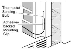
Figure 50 - Locating Thermostat Sensing Bulb on Factory-built Metal Fireplace
